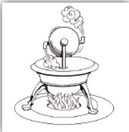
Figure 1. Diagram of an aeolipile. Adapted from reference (5).
